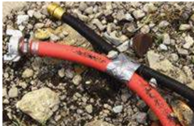
Tape hoses together
