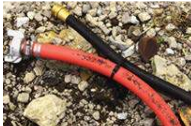
Zip tie or strap hoses together
